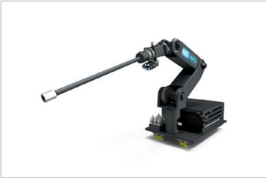
[FilterBot (Primary System Filter Auto Replacement Robot)]
