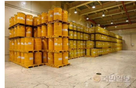
Interim storage of LIRW in NPPs
